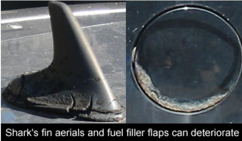
Shark's fin aerials and fuel filler flaps can deteriorate
